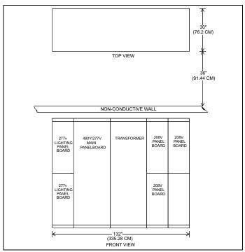
Figure 2. Integrated Facilities Switchboard (IFS).
