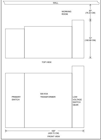
Figure 7. Conventional Secondary Unit Substation.
