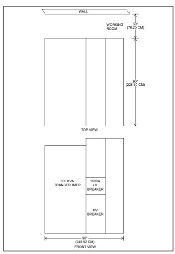
Figure 8. Integrated Unit Substation (IUS).
