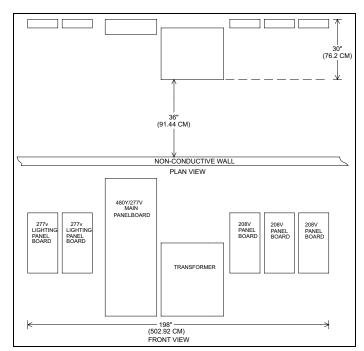
Figure 1. Conventional Panelboard/Transformer Room Layout.
