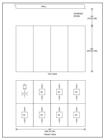
Figure 5. Standard Metal-Clad Switchgear.
