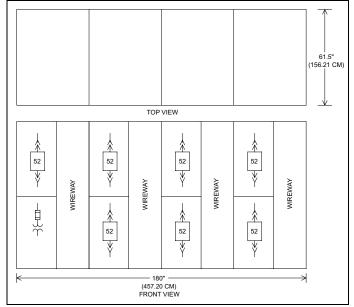
Figure 6. New Metal-Enclosed Vacuum Breaker Switchgear.
