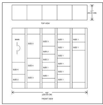
Figure 3. Conventional Motor Control Center (MCC).
